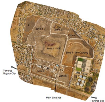
General Contour Survey Ascertains volume of waste
